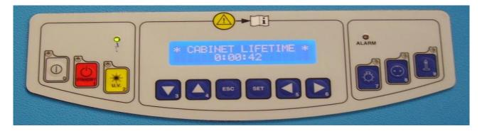
The hour counter starts when the ventilation is switched ON and stop when the ventilation is turned OFF
